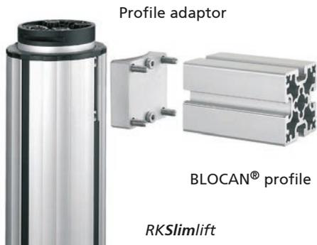
■ The profile adaptor allows several lifting columns to be together to form a stable combination. In this way, and with minimum effort, four columns can be connected to form lifting tables and operated via a synchronous control (MultiControl II quadro). The aluminium profiles F-60/1, F-60-L, F-G 60, F-2G 60 from the BLOCAN® Profile Assembly System are suitable as struts for this purpose.
