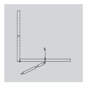
In this position, the point of gravity S is furthest away from the pivot point. The strongest force is required for opening the flap. Both strokes are compressed. The cylinder with the stronger force opens it.
