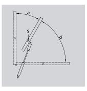
In this position, the point of gravity S moves closer to the pivot point. A weaker spring force is required. Stroke 1 is extended in this position. The spring part 2 with the weaker force now becomes effective.
