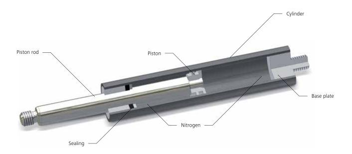
Stabilus gas springs are hydro pneumatic, closed and maintenance-free adjustable elements. The spring force F1 results from the internal pressure in the cylinder, which is generated by the filling medium nitrogen. On the gas spring, this pressure is applied to the cross-section of the piston rod. When no load is applied, the piston rod is always extended.
